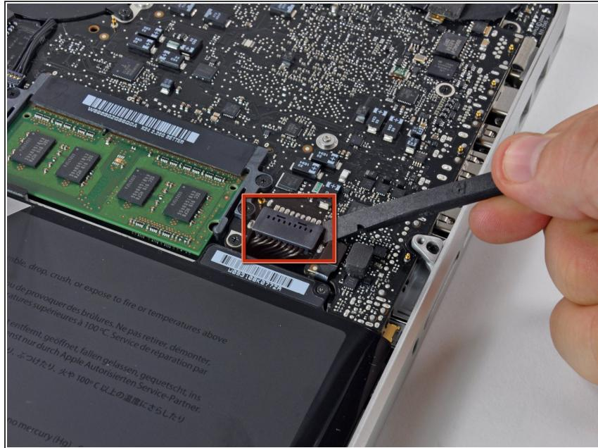
**⚠** For precautionary purposes, we advise that you disconnect the battery connector from the logic board to avoid any electrical discharge.
